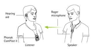
The Roger microphone transmits the speaker's voice into your ears. The system consists of three main elements: Your Naída B-R RIC hearing aids, the ComPilot II with attached Roger X receiver, and the Roger microphone.
