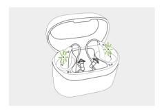
The charging process will automatically stop when the batteries are fully charged, so the hearing aids can be safely left in the charger. It can take up to 3 hours to charge the hearing aids. The charger lid shall be closed while charging the hearing aids.
